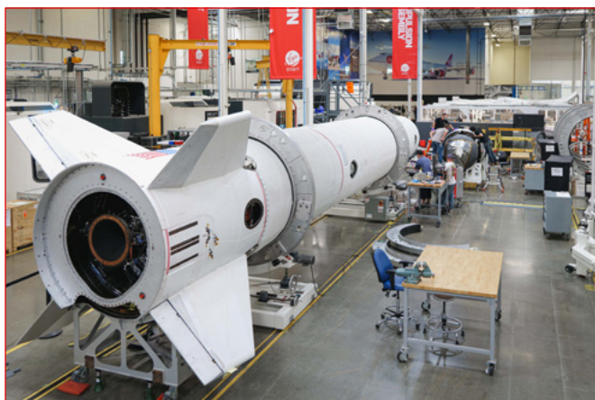
LauncherOne undergoes final integration at Virgin Orbit's manufacturing HQ in Long Beach, CA. March 2021.
